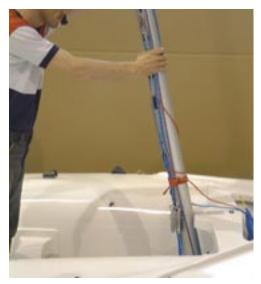
drop it in place. There is a vertical groove in the mast casting and this goes OVER the pin.
