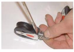
Make sure that the blocks are aligned fore and aft then lock them in that position. They usually leave the factory fully swivelling but there is a small, flat, red locking tab which can be pushed across the block to lock it on either 90 degree axis.
