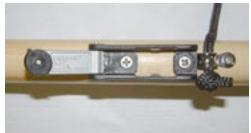
to check the operation, gently pry the cleat open with a flat screwdriver and observe the position of the cam. Also check that the set screw is firmly tightened. - the cam must be held from turning when the screw is tightened. Do not over tighten or you will strip it! Snap back into place.
