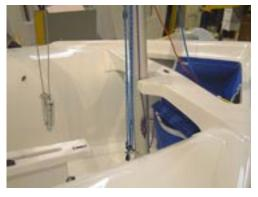
Position the mast in the partner and attach the forestay to the centre pin in the bow fitting. The mast can now
