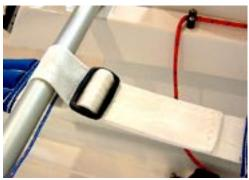
To hold the straps outboard, a line is run from the bridle eyestrap, under the traveller, through the webbing loop then knotted. It can be adjusted.
