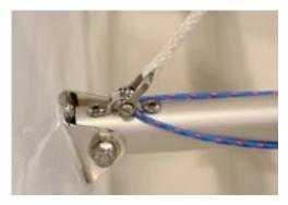
by the yellow hiking strap adjuster rope. One end is tied off at the deck strap. The other goes through the loop in the straps, back through the eyestrap then is tied off on itself in a bowline, Adjust this end of the line for height because the other has the topping lift shockchord retractor attached to it. See bottom picture.
