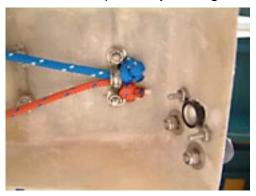
This picture shows the vang (blue), and the c/b downhaul (red), sharing the deckstrap under the cap.
