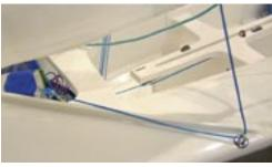
end is rigged, typically, outside the jib, through the guy hook, then to the spinnaker head in the bag.
