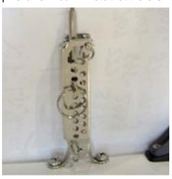
a second pin in the top of the chainplate which must be removed to allow the shroud to pass. Replace this after pinning the shroud as it is a safety device if the main pin happens to come loose (It happens!)
