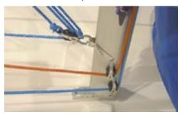
block on the side of the mast. See above. From there it is lead straight back to the aft end of the centreboard cap where it can be cleated off. See following photo. The other
