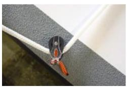
crews prefer to use a continuous sheet with the two ends tied off at the clews. The only disadvantage is that there is always a sheet across the centre of the boat. The sheet is shipped as a single line allowing for this. It may be cut to provide two individual sheets.
