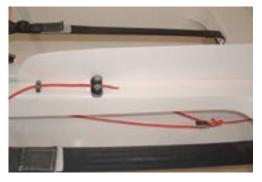
Once through the cap, the end is attached to a single block. A second red line, which is dead-ended under the back of the cap, is then passed through the block and back up through the cap to a CAM cleat. The reason for this type of cleat, as opposed to the Clamcleat is that the rope will run free, unattended, once released and the crew does not have to hold it to keep it from jamming.
