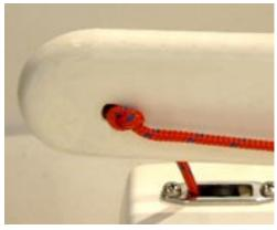
The line is knotted on the other side of the board where it now becomes the uphaul. It then passes down through an exit box in the cap of the centrecase.
