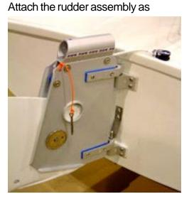
shown. It may be convenient to place the blade in the "up" position and secure there by tightening the black locknut which we have placed on the port side of the rudder head. This may be reversed if the starboard side is found more convenient. Use
