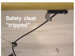
cleat it off. Re-tighten the locknut. If the rudder runs aground or comes in contact with a significant obstacle, the trip cleat will open up as shown in the previous picture.
